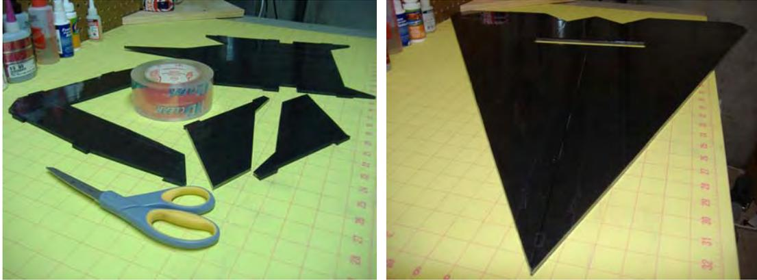
Cut all notches laid out from template on top of main wing. Only cut into top layer of paper and into foam. Remove foam from notches with small screwdriver. Do not cut all the way through other side.
