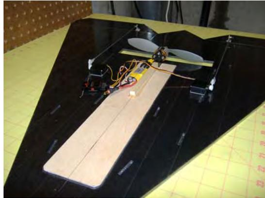
Install all radio equipment and speed controller. Velcro works great for this. Hot glue forward fuselage into notches in wing. Only glue down do one side first then the other side otherwise glue may cool to fast to get fuselage piece into all slots.
