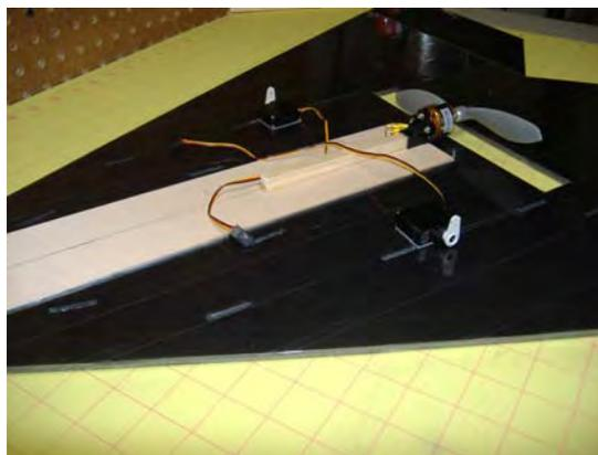
Install servos with double sided tape or hot glue use locations transferred from template. They should be mounted parallel to rear fuselage notch line.
