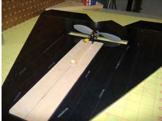
Fit fuselage pieces using bevel and fold technique. Place straight edge ruler parallel with fold line about a ¼ inch away from line. Slide box cutter along ruler angling tip towards fold line. Rotate part 180 degrees and cut the same amount from other side. **Do not** cut all the way through foam board. Remove beveled foam from groove then fold at fold lines. **Do not** glue to wing yet.
