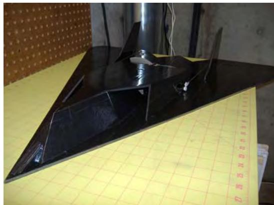
Test the center of gravity with everything on the plane. Slide the battery forward or to the rear till the center of gravity is correct. (Windy) CG is 15.5 measured from front tip of plane back (no wind) 16 inches back.
