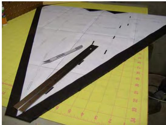
Clear tape all pieces before assembling. This makes the taping process much easier because everything is flat. you only need to tape the outside on the two fuselage pieces. all other pieces should be completely sealed.
