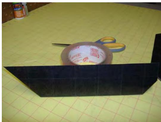
Cut elevator/ailerons (elevons) off the back of wing and bevel bottom of hinge side at 45 degrees or more. Use the straight edge ruler and line it up on top of the edge to be beveled. Holding ruler down firmly, slide box cutter along ruler with tip angled in at 45 degrees or more. Make multiple passes if necessary. Beveled edge must be straight because it will be the hinge point of the elevons.
