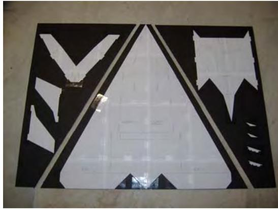
Mark all notches, slots and locations on wing. Mark all fold lines on forward and rear fuselage pieces along with hatch cut lines on rear fuselage. Sit straight edge ruler on patterns and use as a guide to cut out all parts with box cutter.
