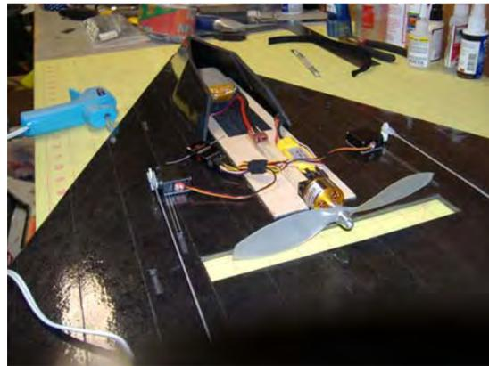
(REVISION) - Build battery box. The battery box makes inserting and removing batteries from plane much easier. Custom fit the box to the batteries you use. Box should be slightly undersize so batteries fit snugly. Glue battery box as far forward as possible or mount with Velcro to help with dialing in CG. Recommend 2200mah Lipos 20c or more.
