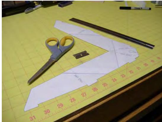
Glue two pieces of foam board together. Clear tape one side to hold pieces together then bend open and apply foam safe CA glue. Lay flat and tape other side while glue dries.
