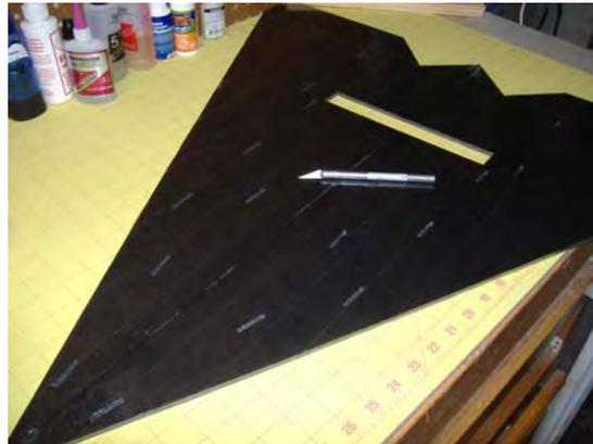
Cut out and assemble the motor stick mount and base plate. Trial fitting everything, then glue mount together with CA glue. **Do not** glue to wing yet. Remove the tape under where the mount will sit by cutting with an Exacto knife or razor. Peel off tape being careful not to tear paper. To minimize this go around the edge of the tape lightly with the razor before removing. Poke small holes into the foam under the mount and scuff the bottom of the wood to provide a more secure bond.
