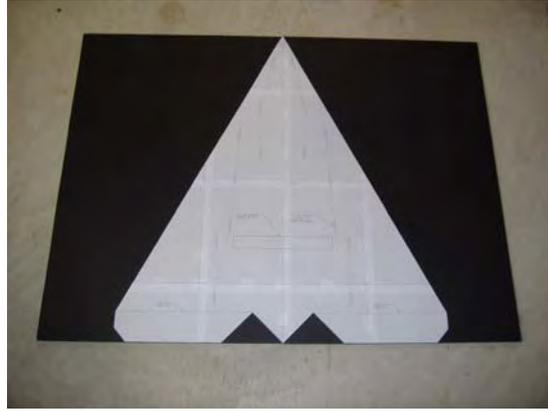
Clear tape the wing, fuselage, tail and nose brace templates to foam board. Use seam on foam board as centerline for wing template.
